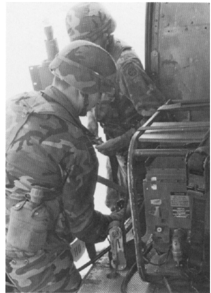
Soldiers secure a PADS in a rear-side cargo compartment of a "Huey" helicopter.
