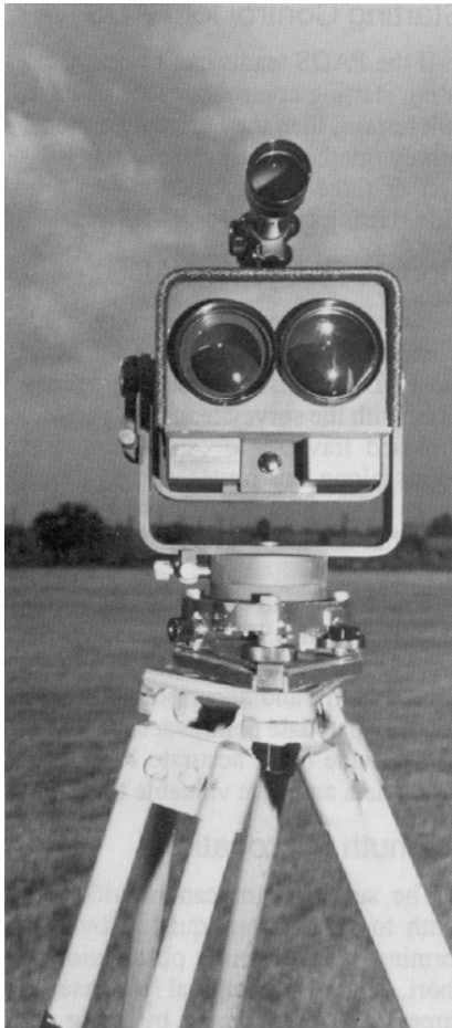
The SEDME-MR measures survey distances up to 7,000 meters.
