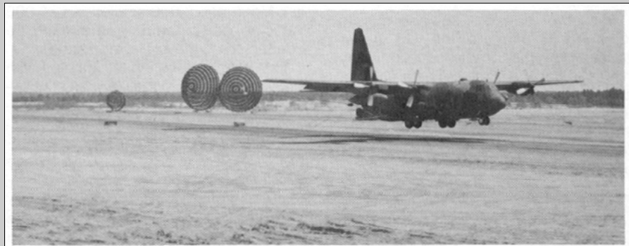
A M198 howitzer from 5-8 FA is delivered to the battlefield using the low-altitude parachute extraction system (LAPES).
