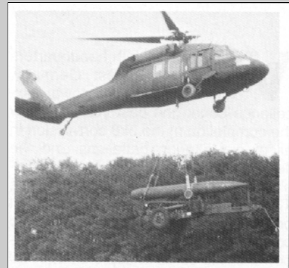
Soldiers of the 42d FA Brigade move a Lance by Black Hawk Helicopter.
