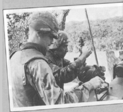
Aiming for accuracy. Cpl Vernon L. Bible (left) checks the setting on his gunner's quadrant while PFC Donnie L. Allen sets the deflection on the Pantel.
