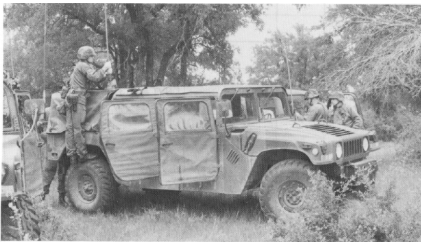
An officer checks to assure his antenna is tightly mounted before his radio is remoted into the TOC.
