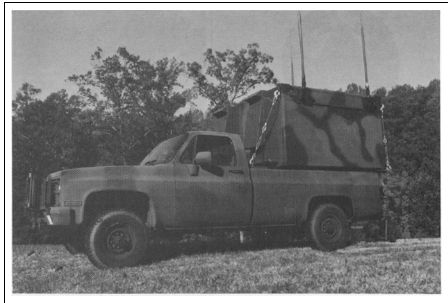
Housed in a shelter mount on a CUCV, the IP automatically tracks and correlates targets using information from multiple sensors.
