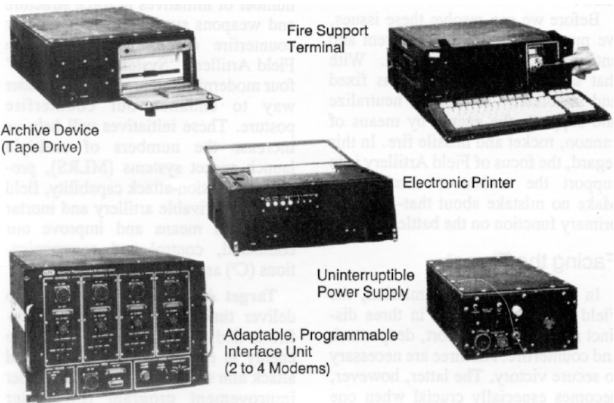
The AFATDS Components for Battery or Platoon FDCs or the Battalion Fire Support Element
