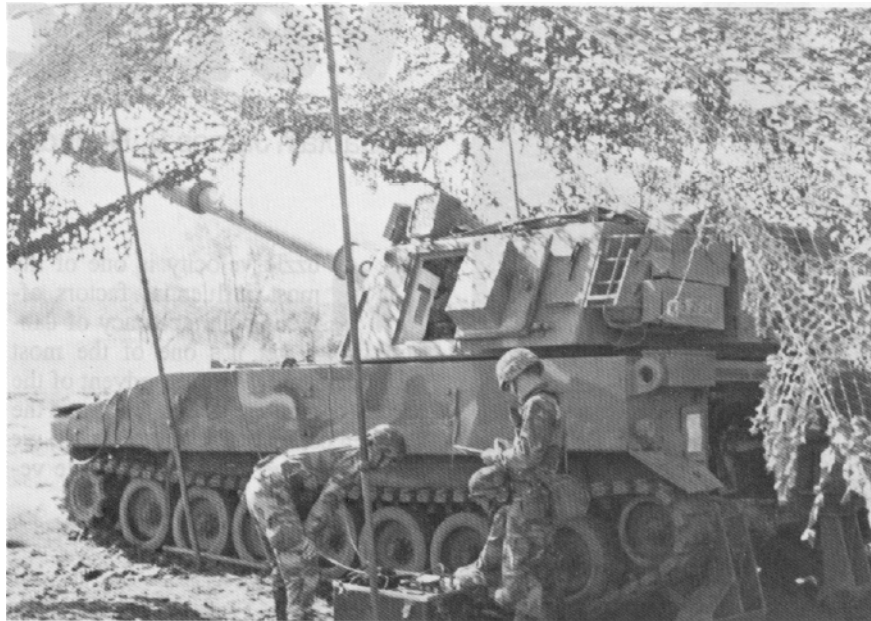
Soldiers record muzzle velocity data from an M90 velocimeter.
