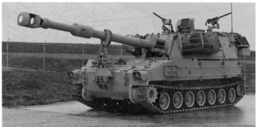
The Israeli M109A1C HIP Prototype, the "Sister" of the US M109A3E2 HIP, Also Under Development
