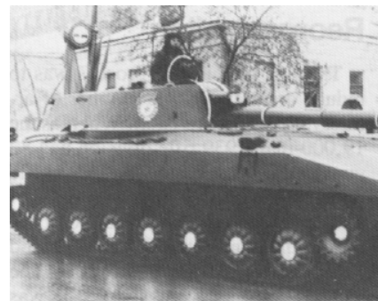
The 2S1 self-propelled, amphibious howitzer, fielded in 1974, is used by the Soviets in Afghanistan.
