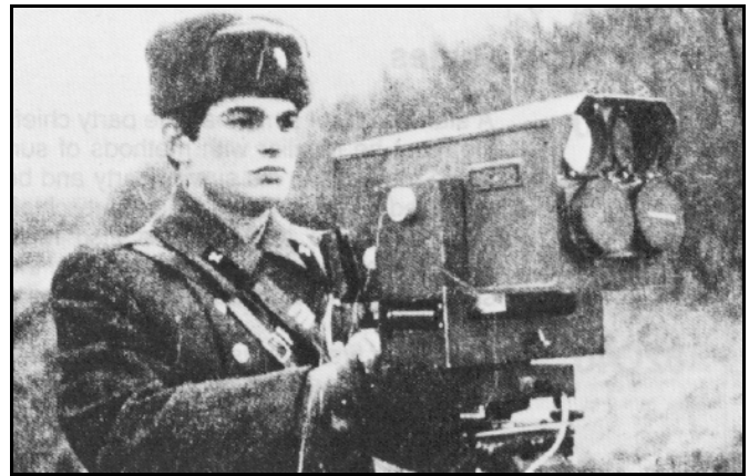
A Soviet artillery lieutenant operates the KTD-1 laser rangefinder.
