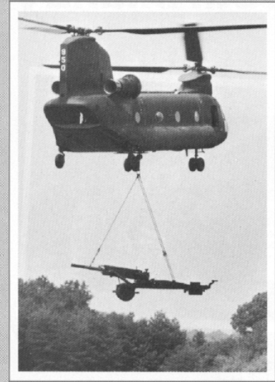
Btry A, 2-110 FA, practices sling-load operations as part of the only RC light IN Div Arty.
