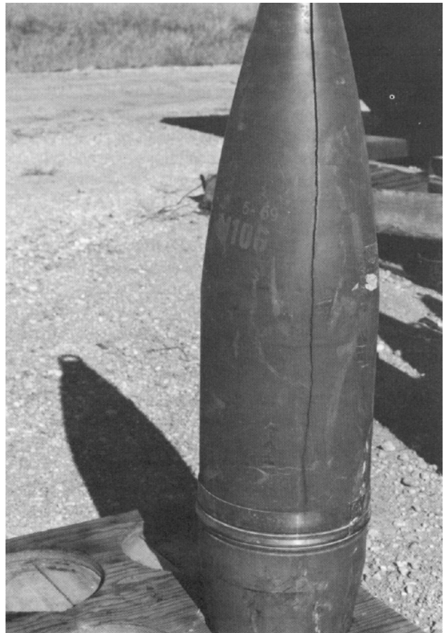
An M106, 8-inch Projectile with a Crack the Length of the Shell Casing.
