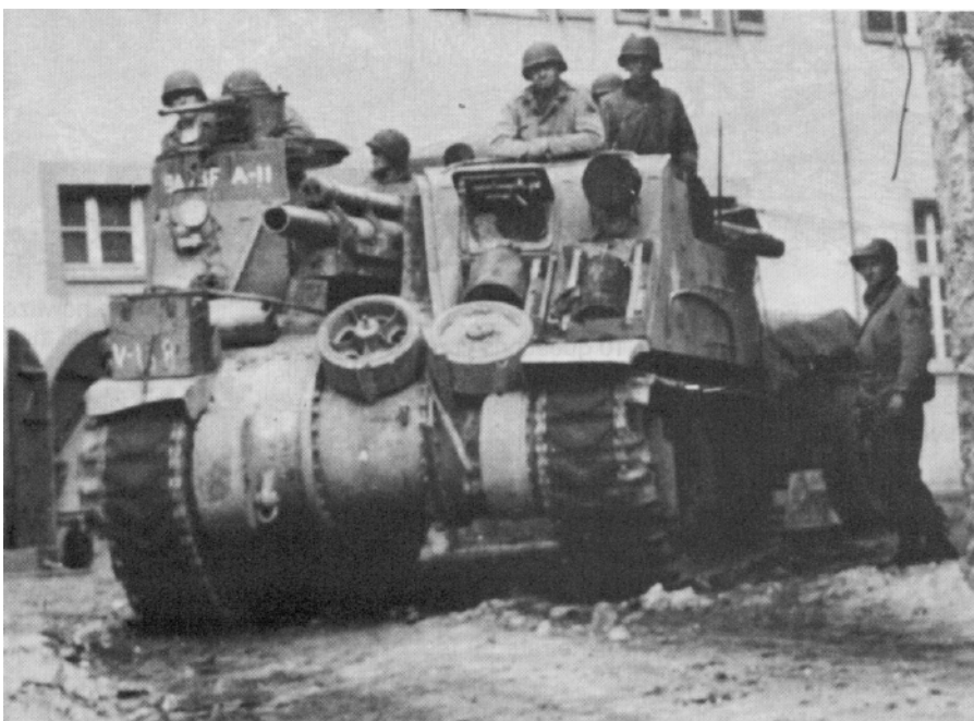
This self-propelled M7, 105-mm howitzer was used for high-angle and direct fire during World War II.
