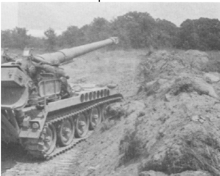
The front end of the howitzer digs into the side of a position that's too narrow as it powershifts.
