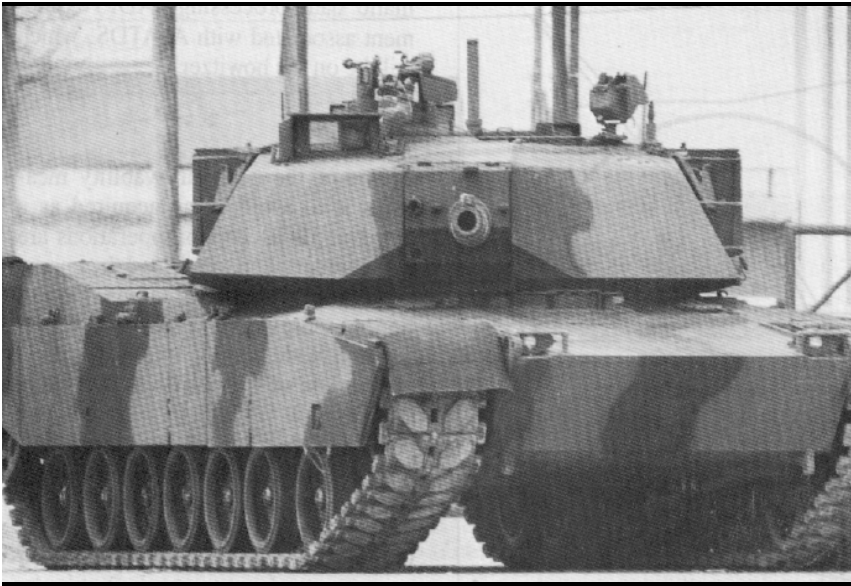
This M-1 "tank," part of the close combat survivability decoy system, is a false target to confuse the enemy.
