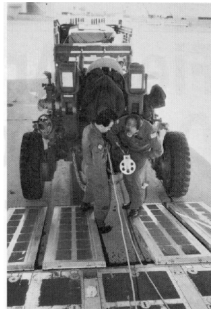
An Air Force loadmaster attaches the C141 winch cable to the chain on the lower carriage of the M198 howitzer to help load the equipment.
