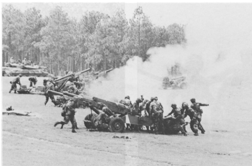
The M102 towed 105-mm howitzer is the backbone of fire support for the light infantry division.
