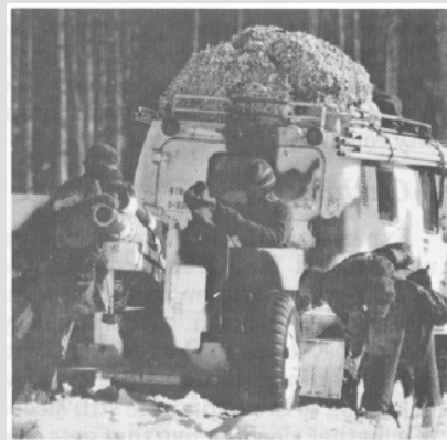
The SUSV's curb weight of 9,790 pounds and maximum towing load of 5,513 pounds makes it ideal as a M101A1 prime mover, ambulance, fire support vehicle, or ammunition carrier.
