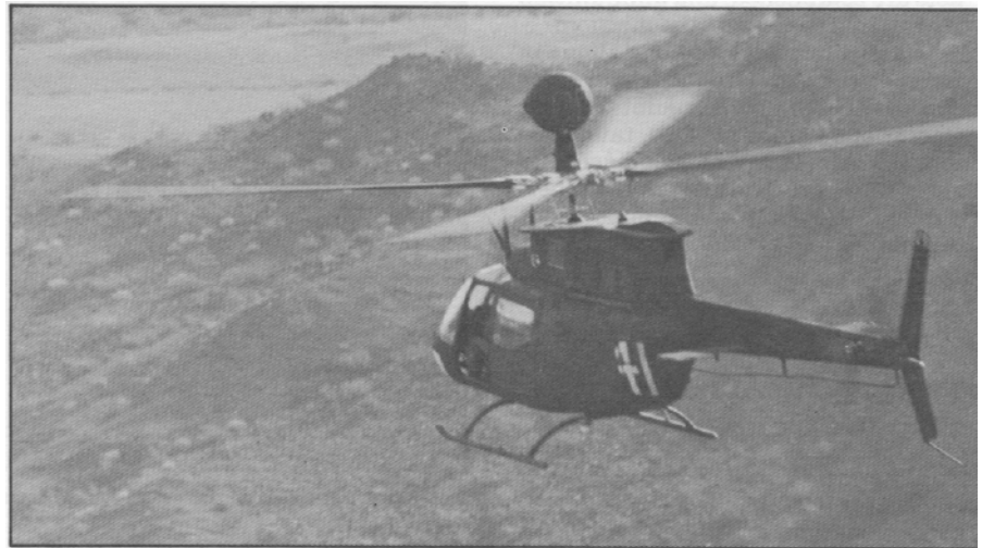
The AFSO can designate artillery fires on the AirLand Battle using the advanced command and control and target acquisition equipment on the OH-58D.
