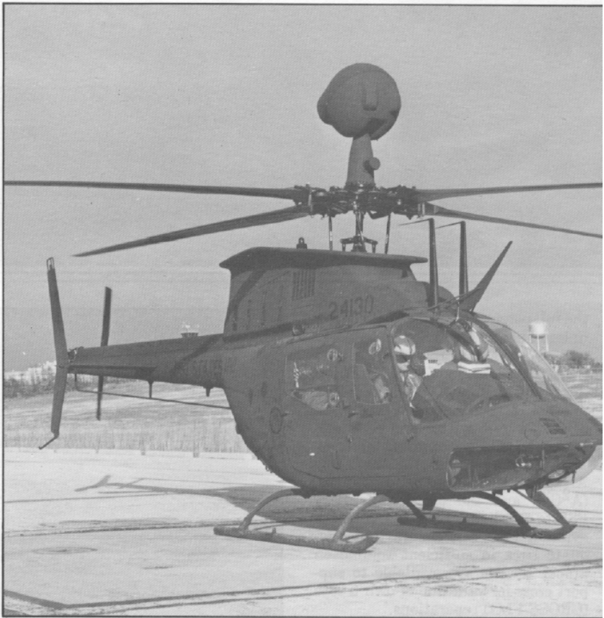
The mast-mounted sight on top of the OH-58D — the Army Helicopter Improvement Program (AHIP).
