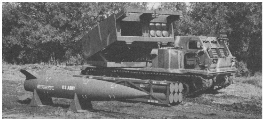
A follow-on development block for ATACMS may include smart munitions to deliver larger payloads to greater ranges than MLRS.
