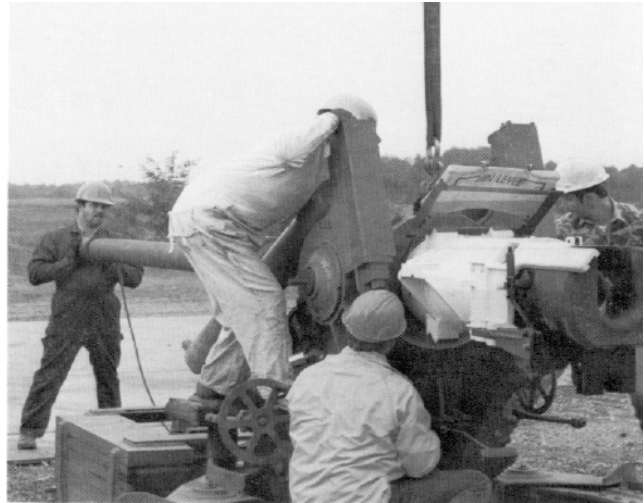
A test crewman uses a power tool to tighten the bolts which hold an M109 cannon assembly on the firing trunnions. The crew needs only 20 minutes to unload a cannon assembly from its flatbed trailer, mount the gun in an M109 turret, proof fire the weapon, dismount the entire assembly, and return it to its pallet on the tractor-trailer.
