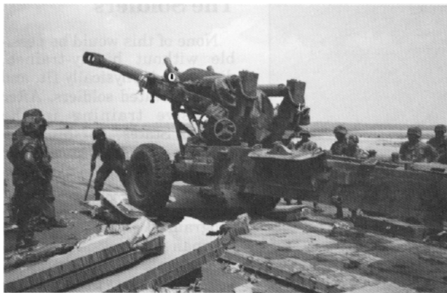
An M198 howitzer completely derigged and prepared for tactical movement following a successful low altitude parachute extraction system (LAPES) operation.
