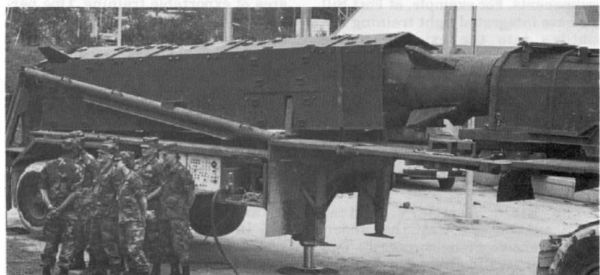
The Pershing II missile requires one-half the time to emplace and displace than the Pershing Ia. The addition of the ballistic shield (bottom) protects the newer system while in transit
