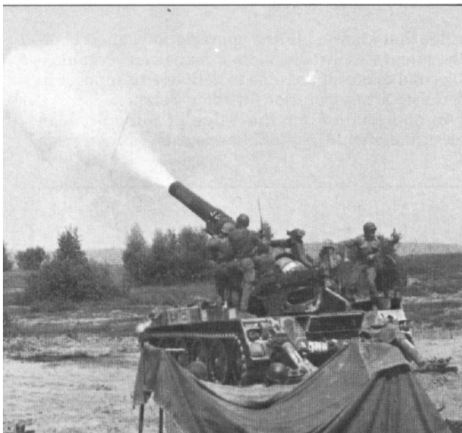
The German artillery possesses a full range of artillery weapons including this general support 203-mm self-propelled howitzer.
