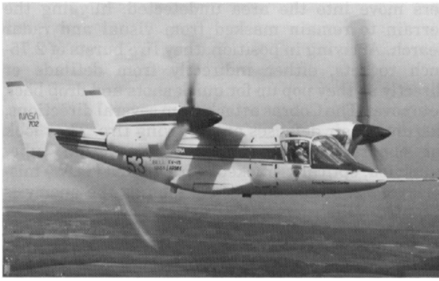
Bell-Boeing's XV-15 tilt rotor research aircraft can convert from helicopter to airplane in just 12 seconds.
