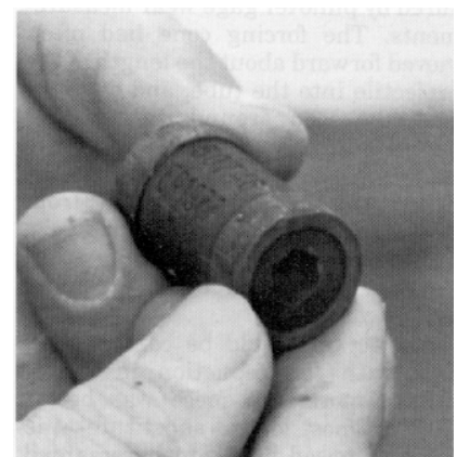
The degree of distortion of a copper sphere within this cylinder enables testers to measure the pressures exerted on a cannon assembly when it is proof tested.
