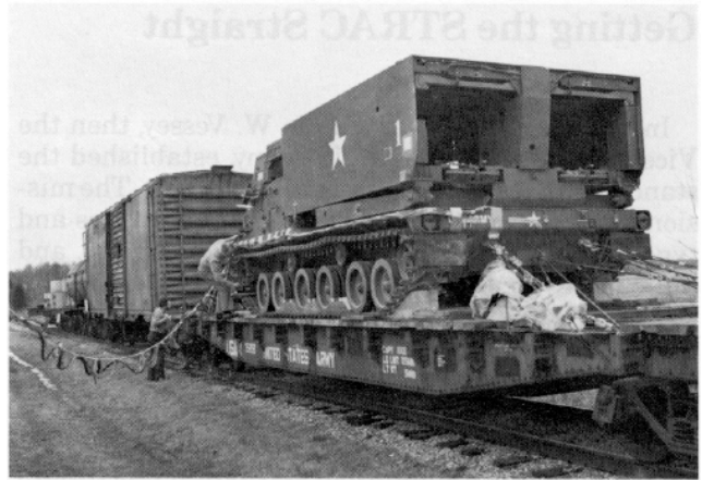
MTMCTEA participated in a rail impact test to ensure that the MLRS would withstand the rigors of rail transport.
