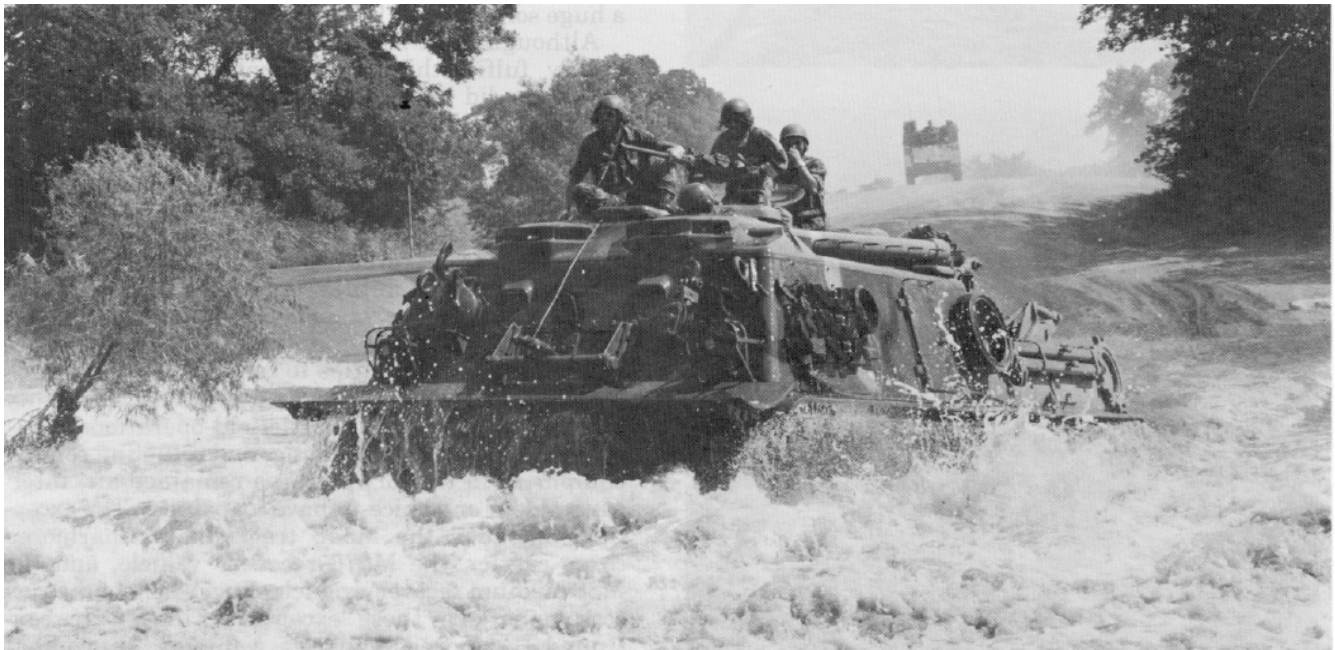
The standard M88A1 is presently in the US' only viable armored logistics vehicle for recovery operations. Eliminating the maintenance function from the list of additional duties assigned to a recovery vehicle increases its ability to perform its primary mission.
