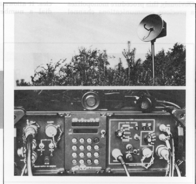
The Erickson MF-15 super-high frequency radio is a highly directional unit.
