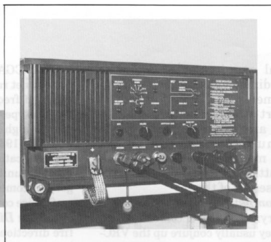
The ER-222 radio is the UHF receiver-transmitter component of the mobile subscriber radiotelephone.
