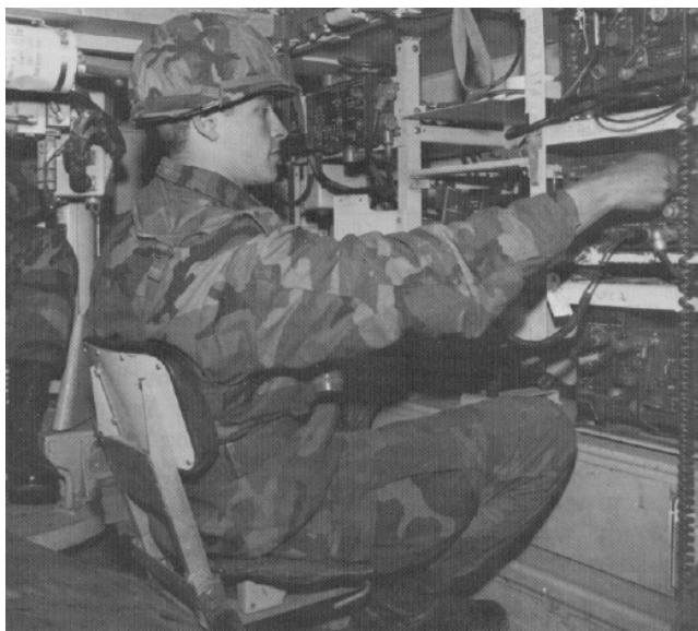
The four-channel intercommunications system and digital message device are used for transmitting fire mission data to a fire direction center.
