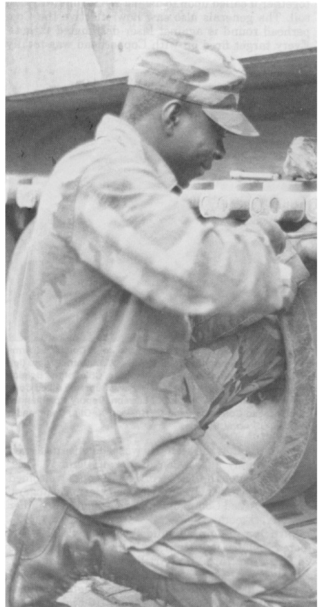
This horse, a 25-ton howitzer, threw some shoes during a 500-kilometer road march from Grafenwoehr. PV2 Tommie Benjamin, Battery C, 4-29th Field Artillery, is replacing one of the 980 pads needed for the 14 tracked vehicles which road-marched back.
