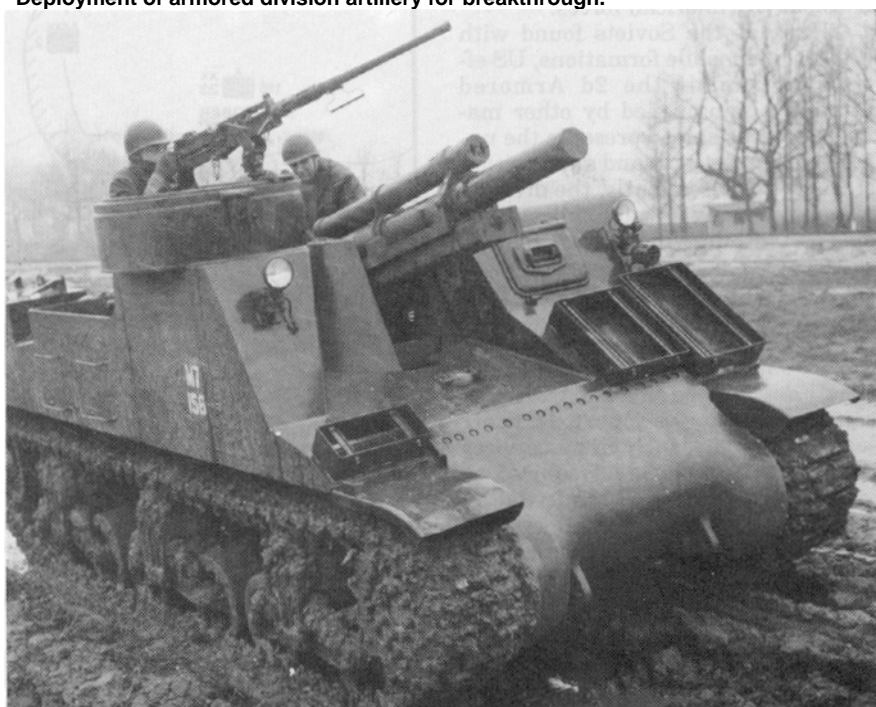
During World War II, division commanders sought to acquire self-propelled howitzers like this M-7 to give mobility and flexibility to their attacking columns.
