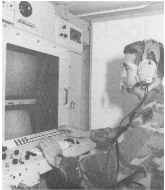
The ground station module is a tactical data processing and evaluation center that links the JSTARS radar to Army command, control, and communications, and intelligence nodes at the corps and division levels. The modules will help commanders perform both battle management and targeting.
