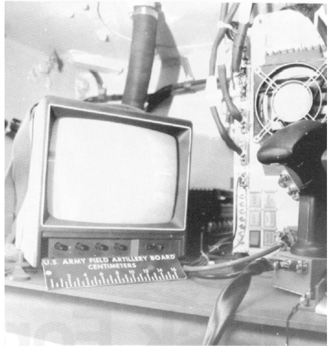
The mobile surveillance system (MSS) internal configuration is a low-light level television which will permit the fire support team vehicle chief to view the battlefield from a buttoned-up vehicle.
