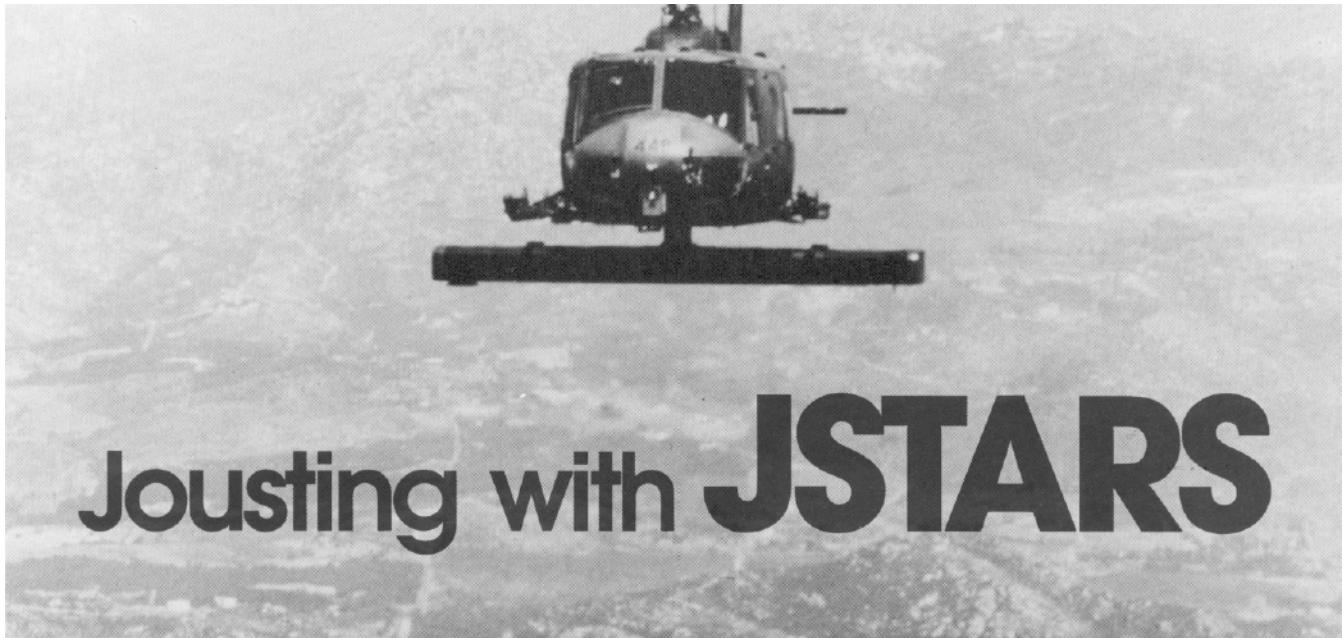
The stand-off target acquisition radar system (SOTAS) is mounted as a rotating "plank" below the main cabin of a Bell UH-1H helicopter.
