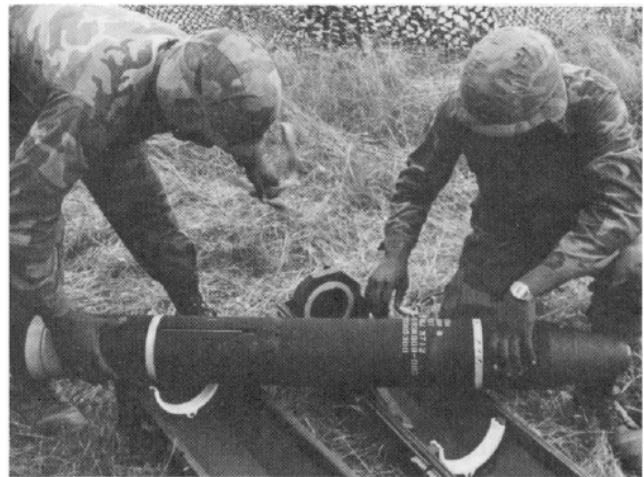
A live Copperhead artillery round gets unpacked for firing by two soldiers from 2d Battalion, 75th Field Artillery, a 155-mm self-propelled howitzer unit from Hanau, West Germany. After being cannon launched and reaching a specific point in its trajectory, the Copperhead deploys guidance fins and glides to a target marked by reflected laser energy.
