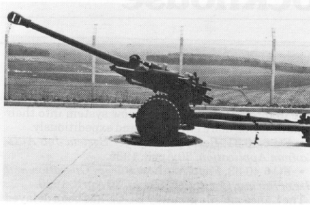
The 105-mm British Light Gun is electrically fired.
