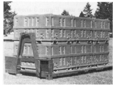
Figure 6. The ammunition module holds 40 complete 155-mm rounds.
