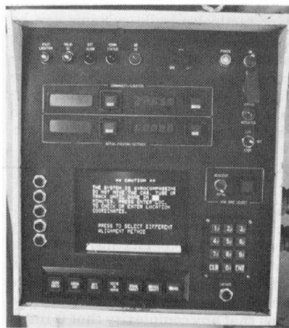
Figure 2. The chief-of-section display console of the test-bed weapon allows the howitzer to work directly with the forward observer.
