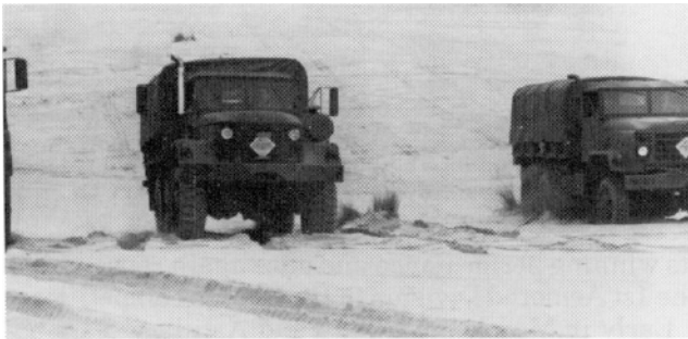
The vehicle on the right is the M923 with single tires and the enhanced mobility system.
