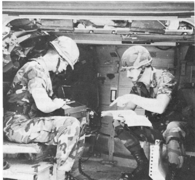
The digital message device can be removed from the mount and hand-held.
