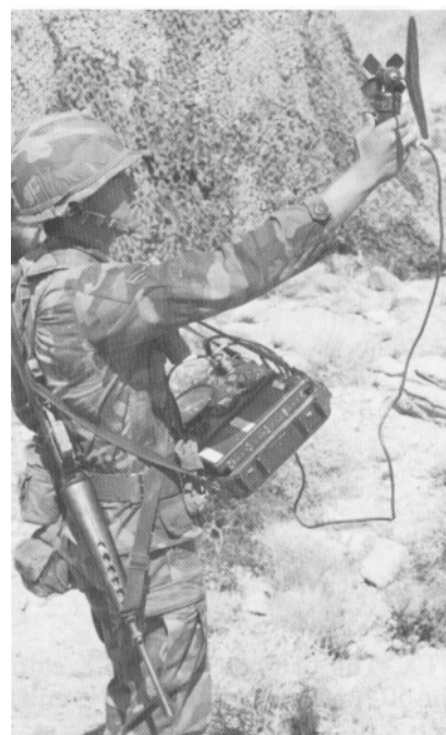
Airman First Class William R. Green, weather observer, uses the TMQ-22 to gather weather data for the soldiers at the National Training Center.
