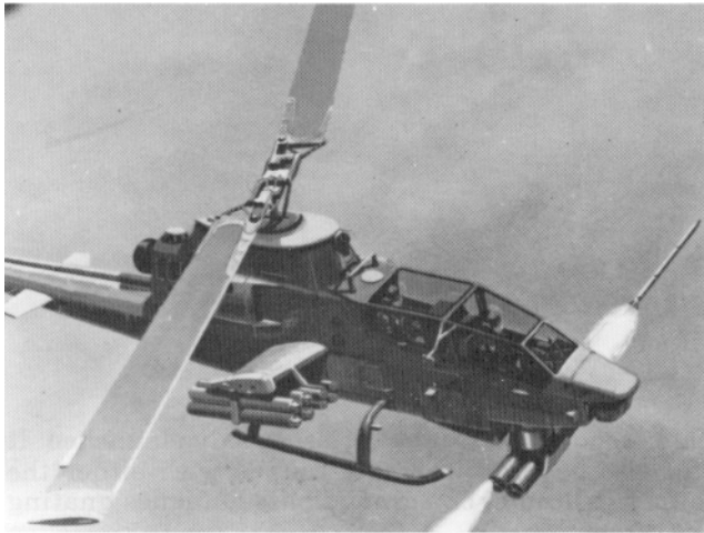
Artist's drawing shows the Spike rocket with multiple penetrator warhead being fired from a helicopter.
