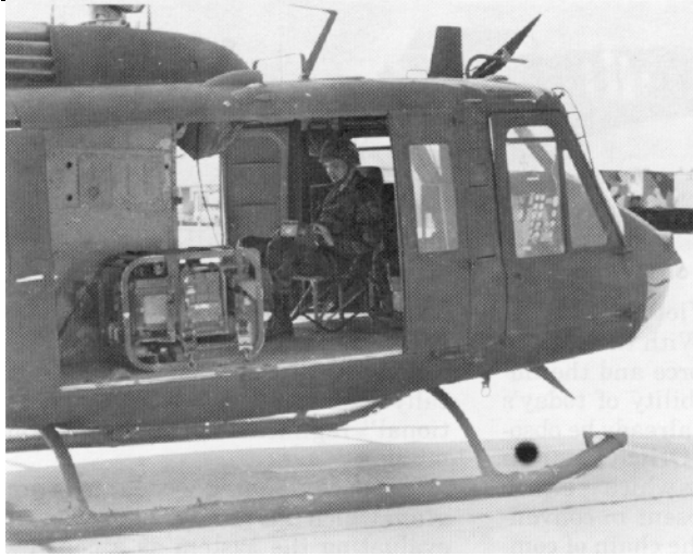
Power for the installed PADS in the Huey is fed from the helicopter through the cable running vertically to the ceiling. The operator is in position on the right. (Photos by SGT James Birdsong)
