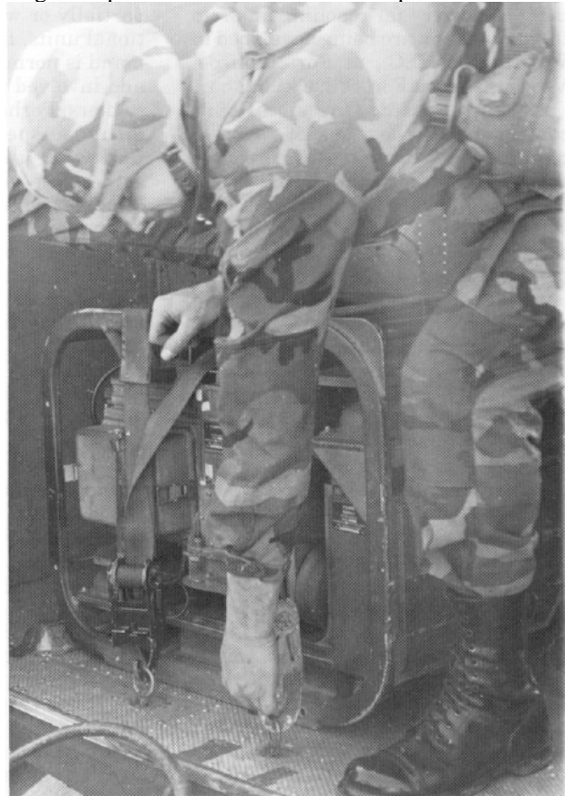
Final tightening of the ratchet straps secures PADS to the aircraft bulkhead.
