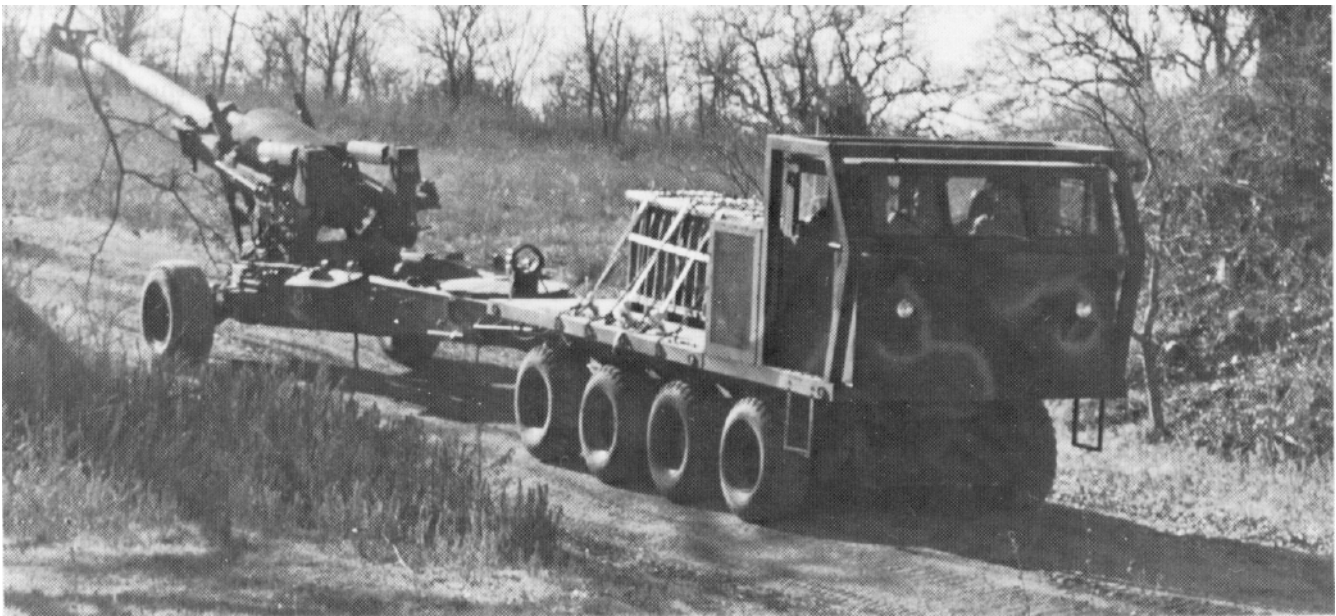
The medium combat truck is being considered as the prime mover for the M198 howitzer and the AN/TPQ-36 and AN/TPQ-37 radar systems.
