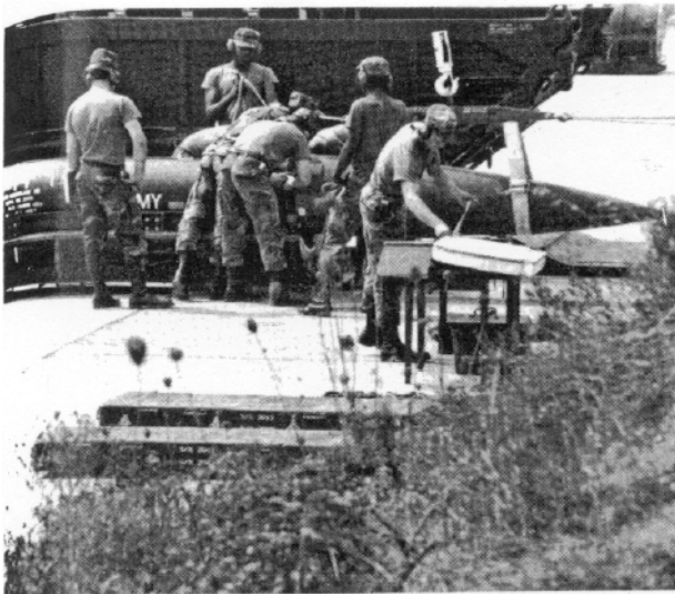
The assembly and transport section carefully mates the two sections of the Lance missile.
