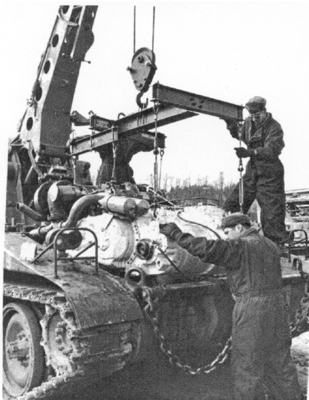
Soldiers from Battery C, 6th Battalion, 37th Field Artillery, replace a power plant on an M578 recovery vehicle. Their battalion was a contender for an Army-wide maintenance award. (Photo by Mark LaMarche)
