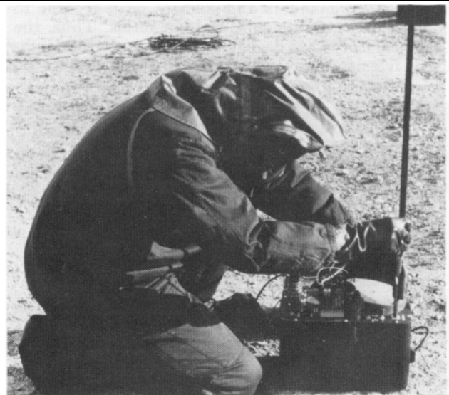
An XM-86 automatic liquid agent detector system is being checked during developmental testing of the device at US Army Dugway Proving Ground, Utah. The XM-86 can be connected by radio to a central alarm as far away as four kilometers. (US Army photo).
