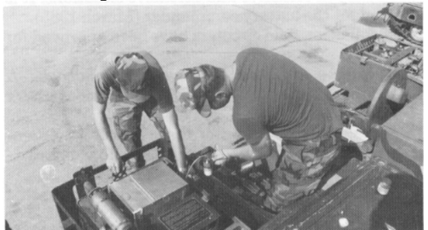
'Skunkworkers' installing a 3-kilowatt generator on an M577.
