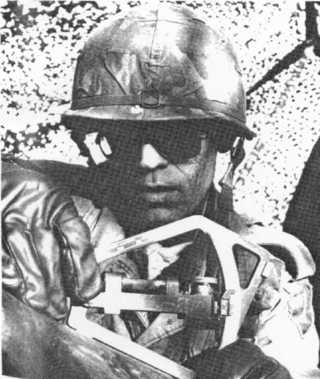
An NCO performs an end-for-end test with the gunner's quadrant during the 2d Battalion, 5th Field Artillery, all-NCO field training exercise.
