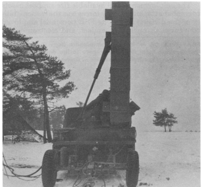
Private First Class Jose Peralta, an AN/TPQ-37 radar operator with Battery C (Target Acquisition), 333d Field Artillery, bore-sights the radar antenna during an 8th Infantry Division (Mechanized) Artillery training exercise. Peralta is one of 11 soldiers who work together as the crew for the Firefinder radar. (Photo by SP4 Timothy Canny)
