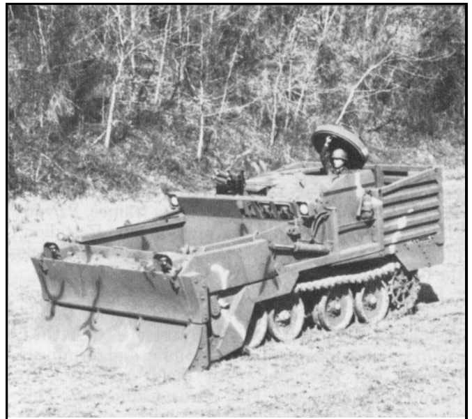
The Army has awarded a contract to produce the first 15 M9 armored combat earthmovers (ACEs). The ACE has a rapid digging capability and is mobile enough to keep pace with the fighting force. It can travel at 30 miles per hour and can be transported in a C-130 airplane and dropped by parachute. The M9 gives its operator protection against small-arms fire, shrapnel, and chemical agents. It can build barriers such as antitank ditches; prepare defensive positions for armored personnel carriers, fighting vehicles, tanks, and artillery; and perform heavy digging tasks to overcome obstacles in its path. Selected combat engineer units are scheduled to receive the ACE in the fall of 1984. (Engineer Update)
