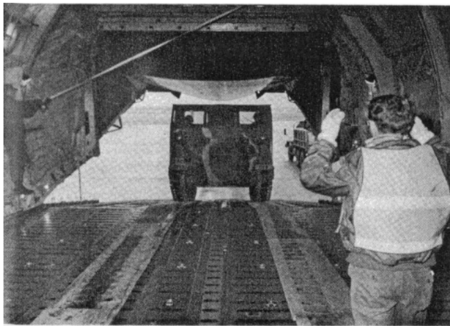
An M548 cargo carrier moves up the ramp of a C-5A on shoring material designed to protect the aircraft floor from damage by vehicle tracks. An Air Force loadmaster guides the cargo carrier into position on the aircraft floor. (Photo by SP5 Mike Howard)
