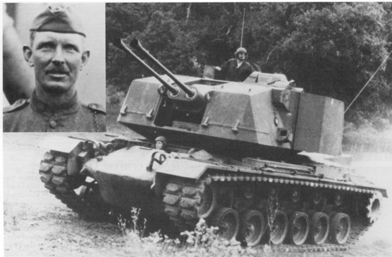
SERGEANT YORK AIR DEFENSE GUN SYSTEM —Named after SGT Alvin C. York (upper left), this air defense gun system roars through recent tests. The Sergeant York has twin 40-mm cannons mounted on an M48A5 tank chassis and features radar-directed fire control. Alvin York, noted for his bravery and sharpshooting during World War I, is the first enlisted soldier for whom the US Army has named a major weapon system. A scale model of the weapon system was presented to Mrs. Alvin C. York at her home in Pall Mall, TN.
