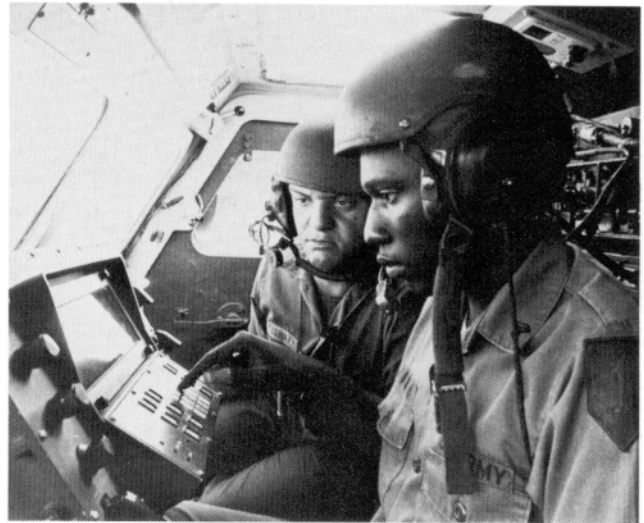
SGT Phillip Battle punches the numbers into the fire direction control panel as SGT Clyde Long watches. The panel is inside one of the platoon's five self-propelled loader/launchers and can communicate to the computer device in the platoon headquarters tracked vehicles.
