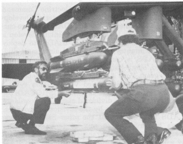
Technicians at Redstone Arsenal load a Hellfire antitank missile onto an ESSS rack during BLACK HAWK/Hellfire missile test.
