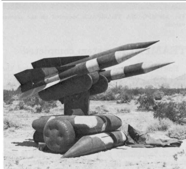
Is it the "Real McCoy"? At a distance the inflatable Hawk missile system decoy passes surveillance test as the real thing.
