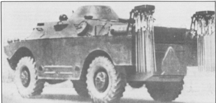
A BRDM-2 rkh (also known as the BTR-40PB rkh) showing at the rear of the vehicle the marker flags which can be fired into the ground to mark safe lanes or contaminated areas. This vehicle also carries a GSP-11 automatic chemical-agent detector-alarm and a PPKhR chemical-agent detector. These are mounted externally on the superstructure just above the right rear wheel arch. When not in use, the flag pickets and firing devices are wrapped and stowed on each side of the rear hull roof of the vehicle.
