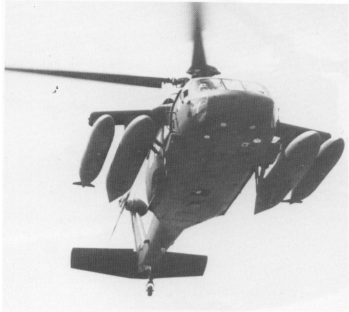
The External Stores Support System (ESSS) being developed for the UH-60A Black Hawk helicopter will provide a self-deployment for the aircraft when equipped with two 450-gallon tanks and two 230-gallon tanks.
