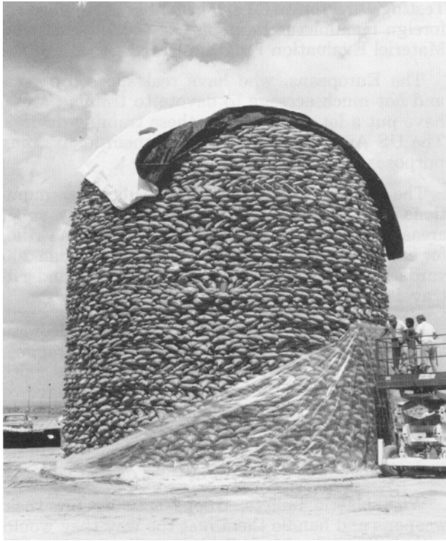
Engineers inspect nearly 600 tons of ammonium nitrate fuel oil (ANFO) before placing it into firing position. The resulting explosion resembled a giant mushroom cloud reminiscent of a nuclear fireball.
