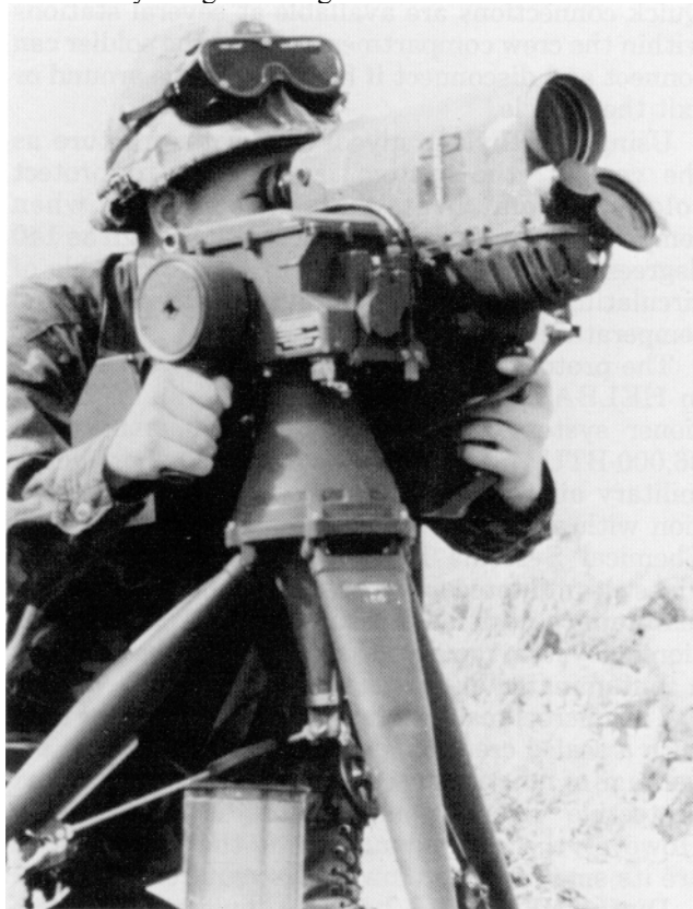
A US Marine sights a target with Modular Universal Laser Equipment (MULE) during rugged operational tests of the laser device.
