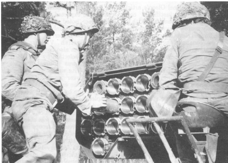
Reloading and loading is done by hand. A well-trained crew can reload all 36 tubes in 20 minutes.
