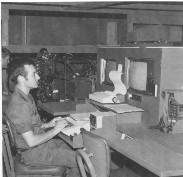
Targeting Cell console with microcomputer, A&B scopes, and TACFIRE VFMED mounted in a 5-ton expansible vehicle.
