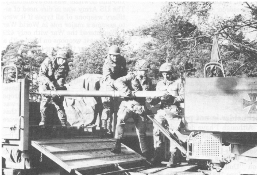
Off-loading the rockets from the 10-ton support vehicle. This truck can carry 180 rockets.
