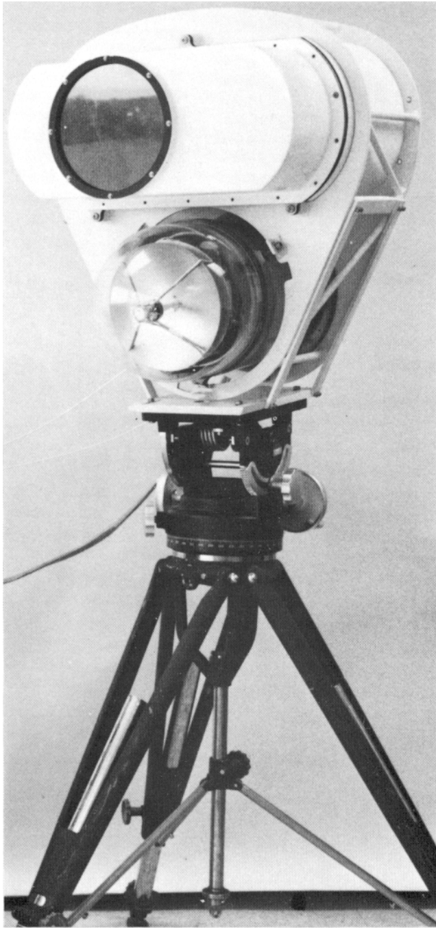
Figure 4. Millimeter wave seeker.
