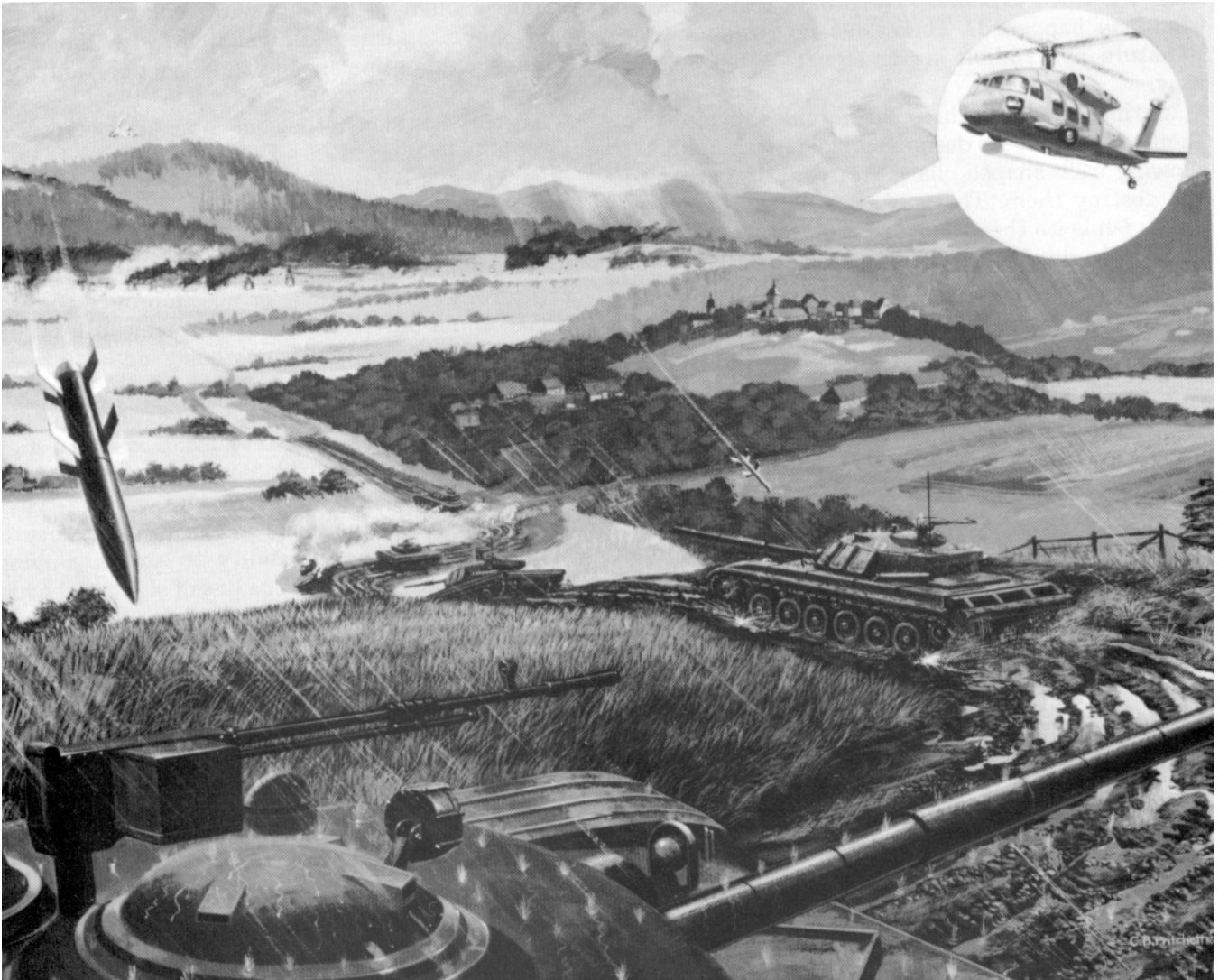
Figure 2. An artist's concept of the Advanced Indirect Fire System and Stand-Off Target Acquisition System (insert at upper right), showing the infrared round (lower right) and the millimeter wave round (lower left) about to strike target tanks.
