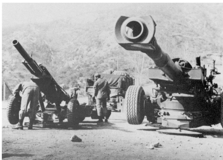
The M198 155-mm howitzer replacing the smaller 105-mm howitzer in the 2d Infantry Division weighs 4,850 pounds.
