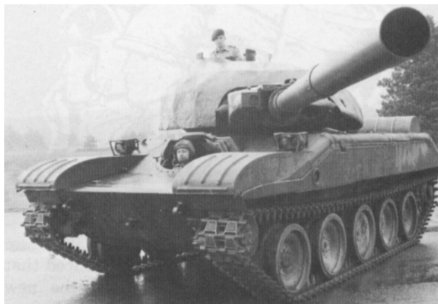
SGT Bruce Meier and SP4 Roscoe Shepherd, 9th Infantry Division Opposing Forces Detachment, drive this Russian-looking tank into the division headquarters parking lot for display. It's an M551 Sheridan inside the shell of a Soviet T-62 mock-up. (Photo by Scott Davis)
