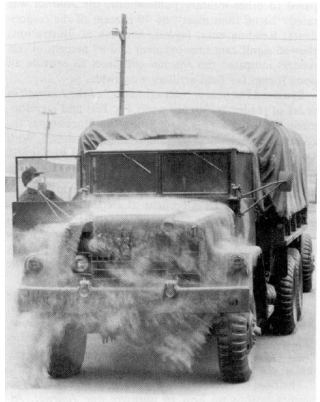
The coarse ash clogged air filters and eroded brake drums on vehicles.
