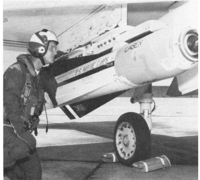
US Marine Corps Major John P. Bland inspects an AGM-65E Laser Maverick mounted on an A-4M attack aircraft prior to the test flight in which he launched the air-to-surface missile in the first firing of a Maverick by a Marine Corps pilot and the first from a Marine aircraft. The recent low-altitude, long-range launch scored a direct hit on an armored personnel carrier target at Eglin Air Force Base, FL. This was the third launch in succession of the AGM-65E to score a direct hit. The missile is a laser-guided version of the US Air Force's Maverick with a heavier warhead. The air-to-ground weapon is being developed by Hughes Aircraft Company under an Air Force contract primarily for use by the Marine Corps for close air support of combat troops.
