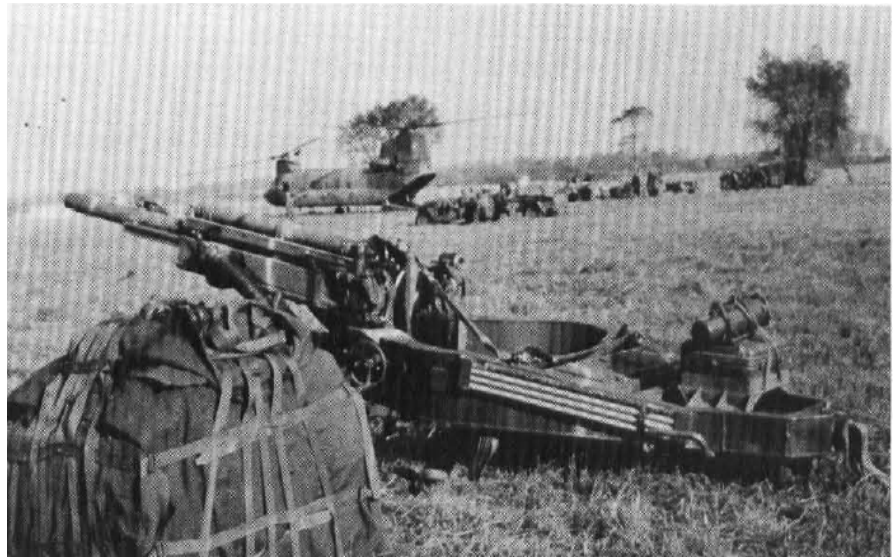
Figure 6. An M102 howitzer with A-22 bag rigged for external sling loading. (Note spacing between loads.)
