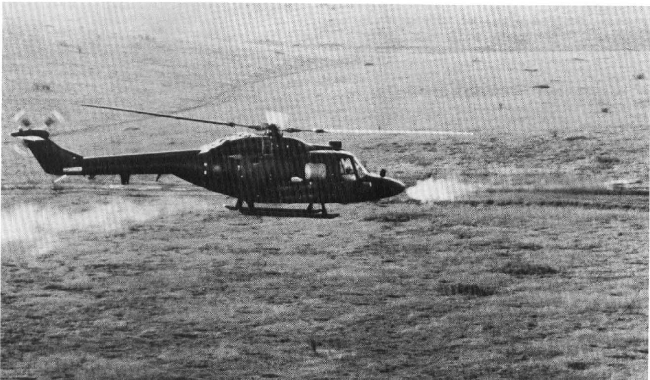
TANK TRACKER — A TOW antitank missile is launched from a British Army Lynx helicopter during recent firing trials. Under a Ministry of Defense contract, British Aerospace Dynamics will produce the airborne TOW system under license from Hughes Aircraft Company. TOW, the tube-launched, optically-tracked, wire-guided missile system developed by Hughes for the US Army, has been deployed with the air and ground forces of 30 other nations.
