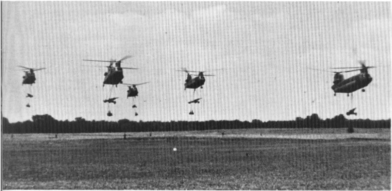
Figure 5. The simultaneous movement of battery loads requires sufficient spacing in the pick-up zone.
