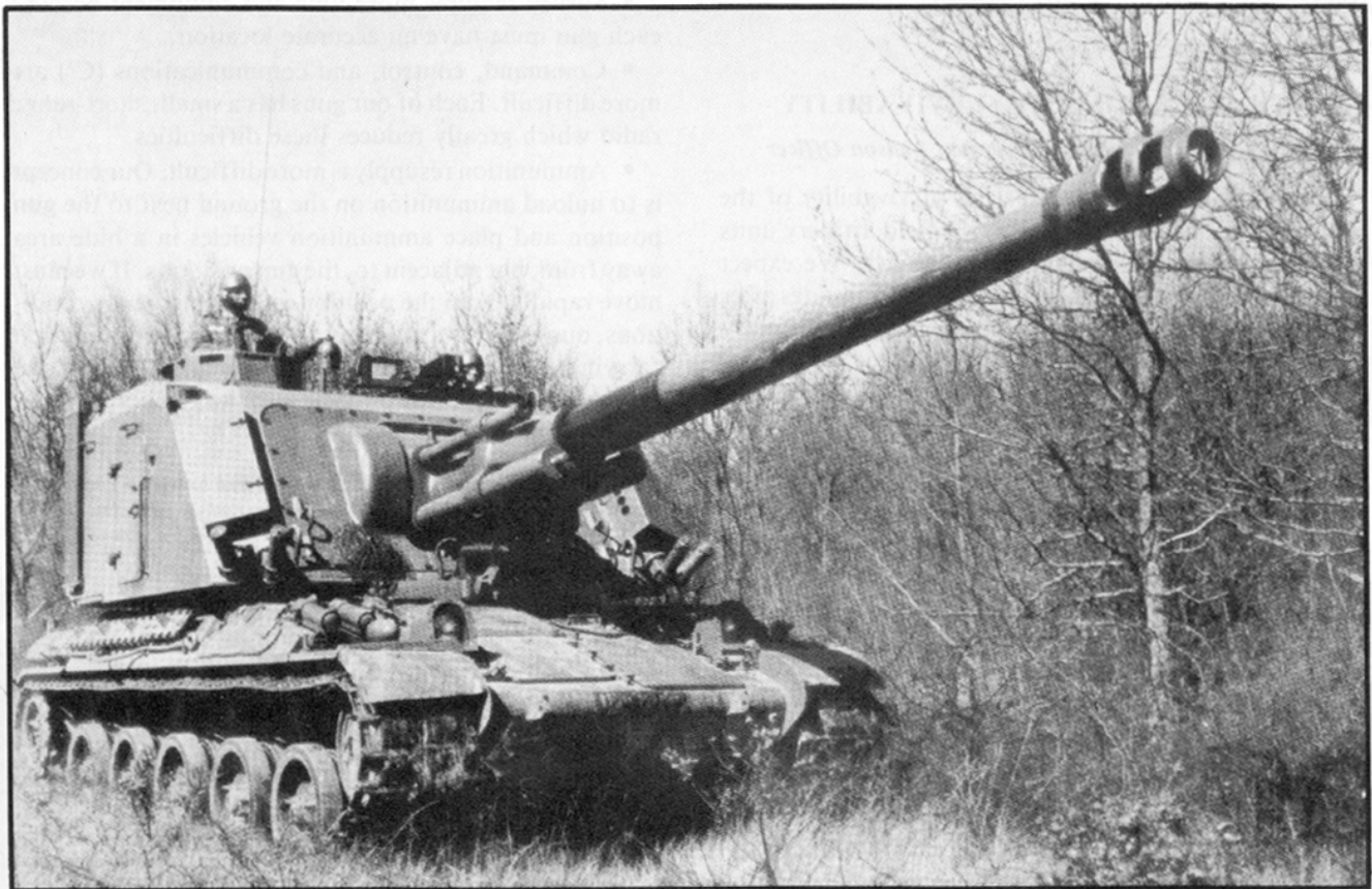
Figure 6. The French 155-mm automatic loading howitzer, firing a standard projectile, has a range of about 24,000 meters.
