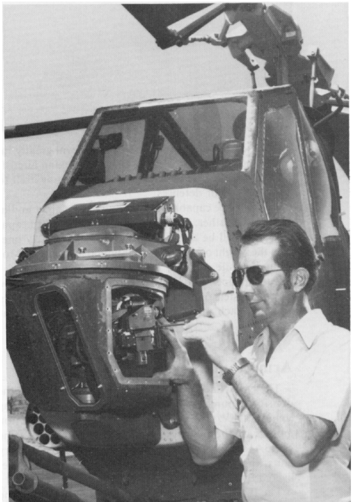
Technician installs the telescopic sight (equipped with mini-laser rangefinder) in the Cobra helicopter. (Hughes photo)
