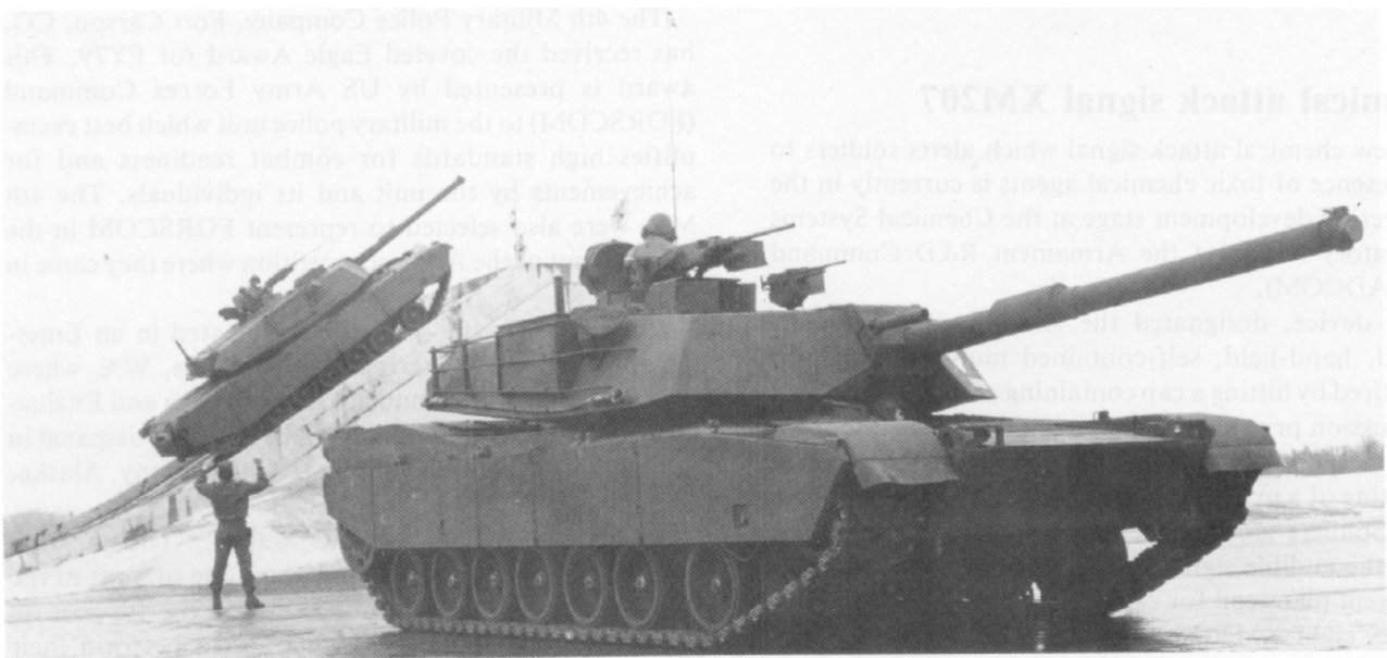
The XM1 Abrams tank. On the left, the tank is demonstrating its vertical climbing ability.
