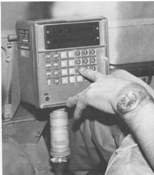
The Control and Display Unit (CDU).
