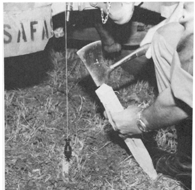
PADS operator prepares to install a stake for the battery center.
