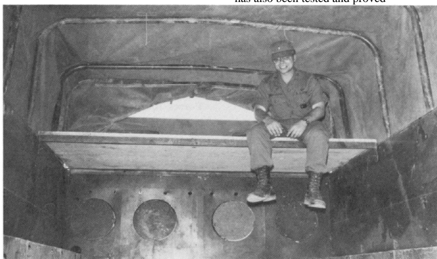
Figure 3. Balcony in M548 for storage of TA-50.
