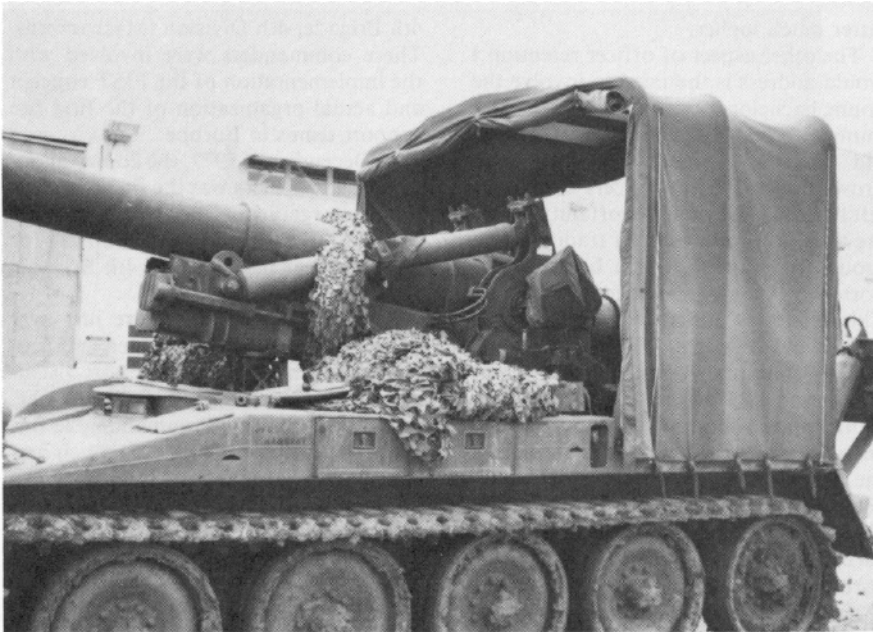
Figure 4. M110A1 fabricated winterization kit with front curtain rolled up. Side curtains will also roll up, and top provides storage for camouflage net in transit.
