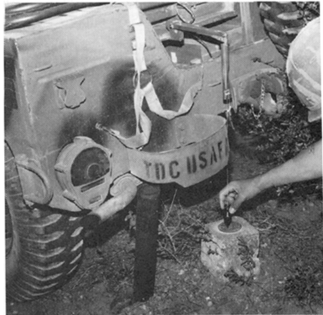
The PADS operator updates the system by precisely locating it over a known survey control point.
