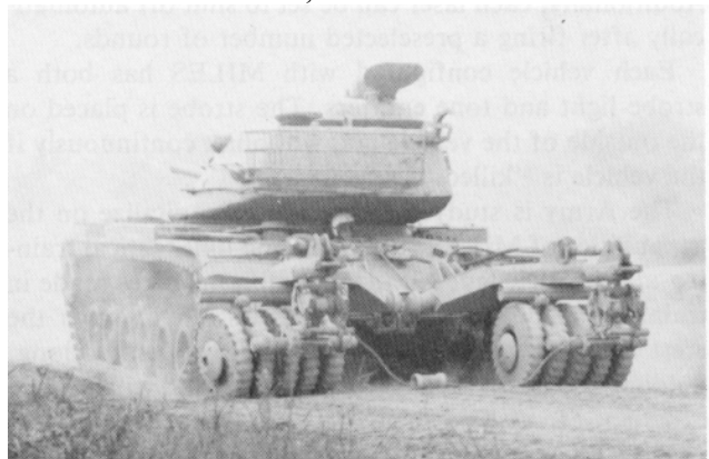
The Army's new mine clearing roller system mounted on a tank.
