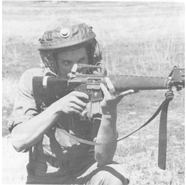
PVT Donald L. Stewart of CDEC's Armor Company C demonstrates the MILES infantry harness assembly. The laser, mounted on the barrel of the M16 rifle, can be set to fire a predetermined number of times and then shut itself off. (Photo by Bob Hubbert)
