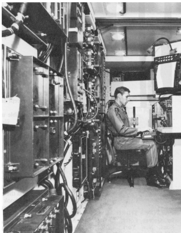
TACFIRE goes beyond the earlier modeling of ballistic trajectories. This Litton-built, third generation machine digitally models the broad battlefield situation leading to, and including, ballistics.
