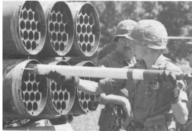
M200 rocket pods armed with 2.75-inch folding fin aerial rockets are possible aids in both antitank and air defense of the battery area. (Photo by David Sleeth)
