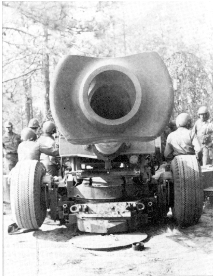
You're looking down the business end of the M198 as a crew from the 1st Battalion, 73d Field Artillery, prepares to "get 30" kilometers. Note the protective helmets and the base plate which helps the crew traverse the 15,000-pound howitzer. (Photo by Charles Ray)
