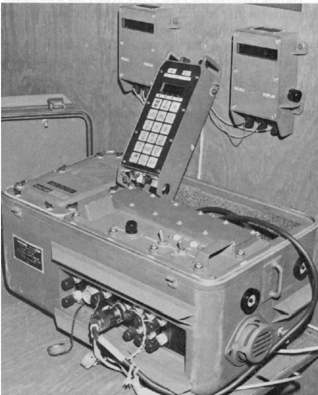
Figure 2. The Gun Display Unit includes the Section Chief Assembly, two identical Gun Assemblies, and a carrying case.
