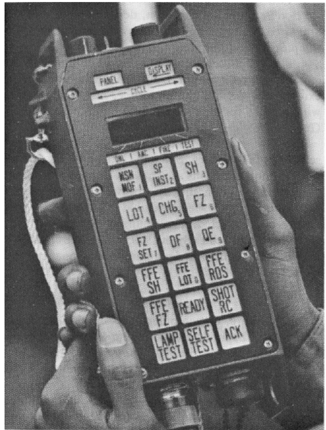
Figure 3. The cycle buttons on the Section Chief Assembly allow the section chief to display fire commands. Pushing any button on the front panel causes that element of the fire command to be displayed immediately. A connector allows a headset to be attached for voice communications.
