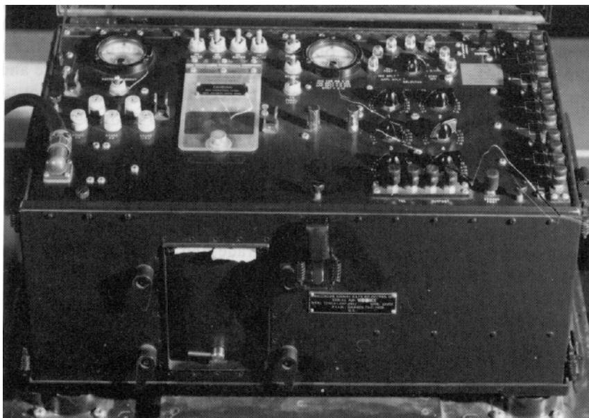
Sound ranging sets from World War II and today show the changes in equipment. The GRS-3 (top), shown in the back of a ¼-ton truck, has been replaced by the TNS-10 (bottom) which is being issued to sound ranging sections.
