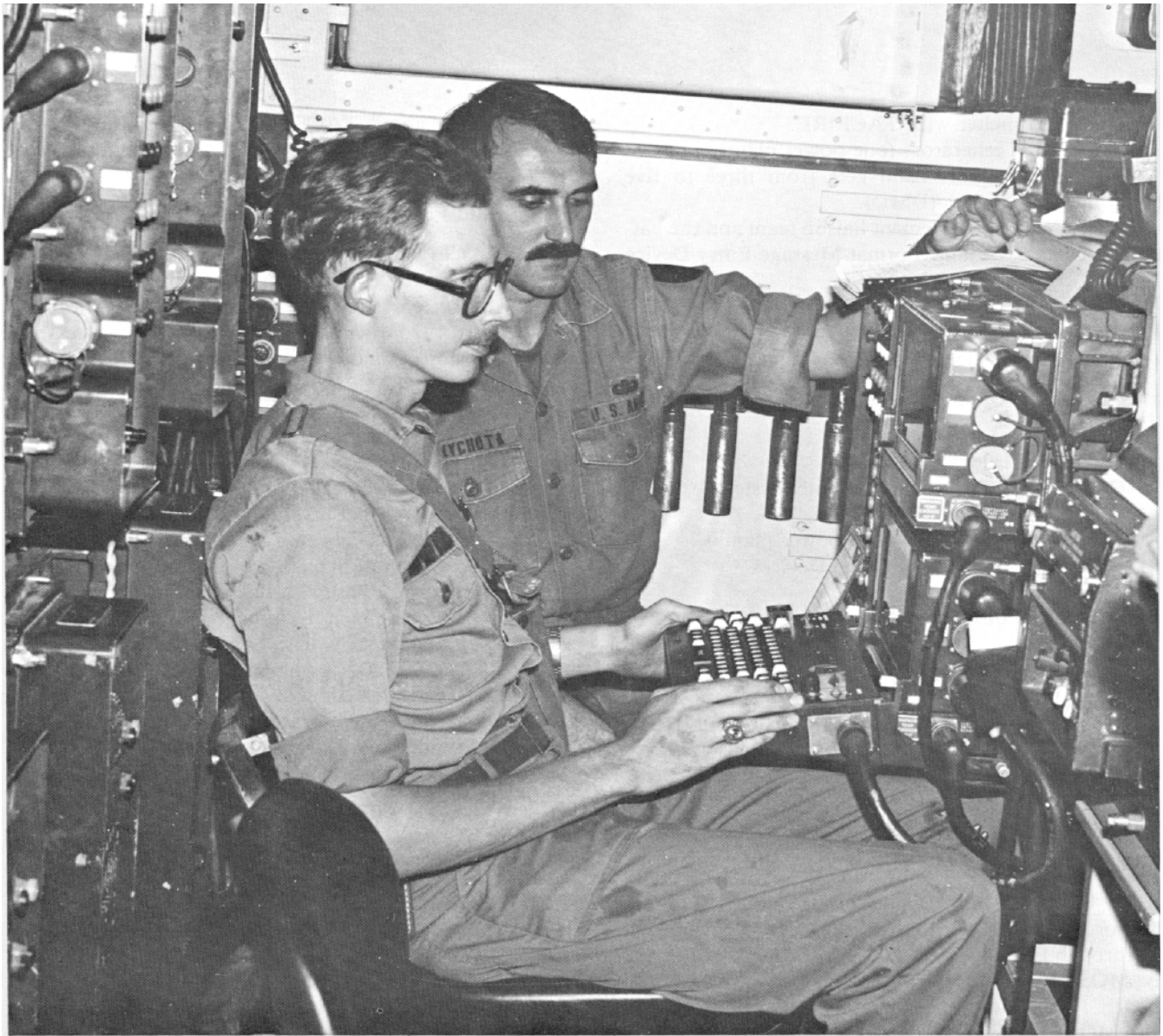
A fire direction officer and fire direction sergeant are seated at the Artillery Control Console of a Field Artillery battalion TACFIRE set.
