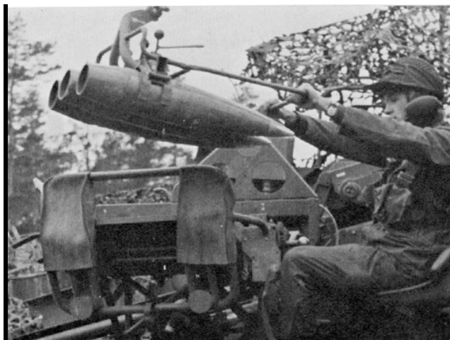
The loader, one of only six crew members, guides three projectiles to the loading table. This system permits a burst rate of fire of six rounds in 20 to 25 seconds.
