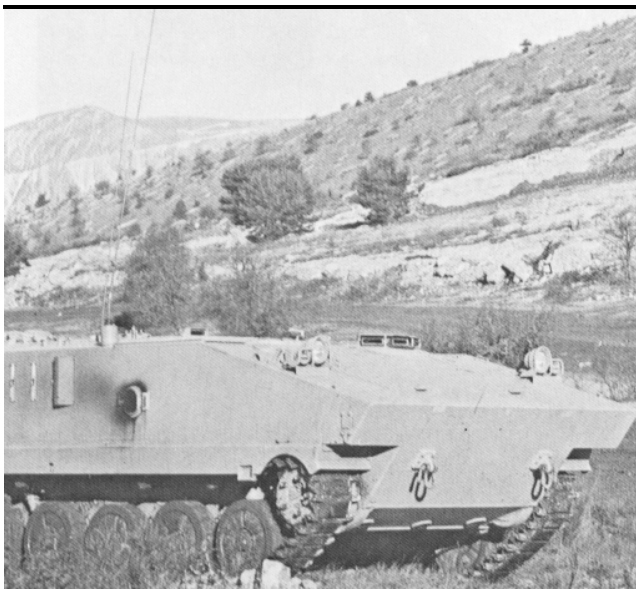
"Atila" is the name given this very low profile vehicle used for fire direction centers and command post operations.
