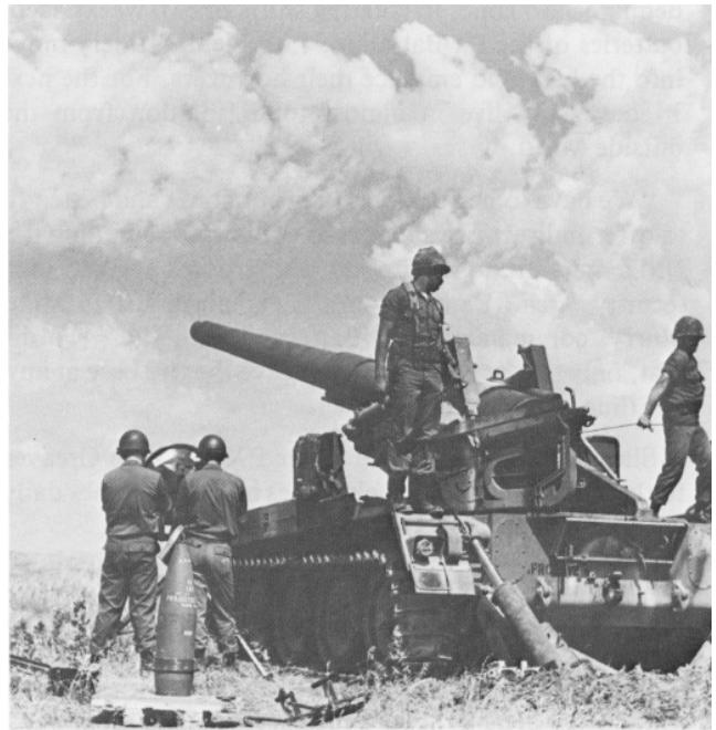
FORT SILL, OK — The instant between pulling the lanyard and firing the round is caught as soldiers of the 2d Battalion, 12th Field Artillery, fire the first test rounds through the recently modified M110 8-inch howitzer, now the M110A1. The battalion is the first TOE unit at Fort Sill to receive the improved howitzer. Modifications are explained on page 43 of the May-June 1978 Journal. (Photo by SSG Ron Hatcher)
