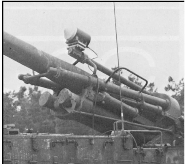
Calibration and measurement of muzzle velocity is accomplished with the "Miradop," shown here mounted on an obsolete weapon.
