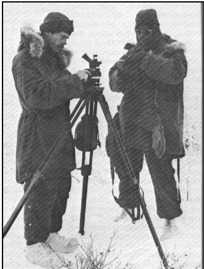
Personnel must be careful not to breathe on the optics of the aiming circle. At these temperatures, the moisture from a person's breath immediately forms a coat of ice on a lens.
