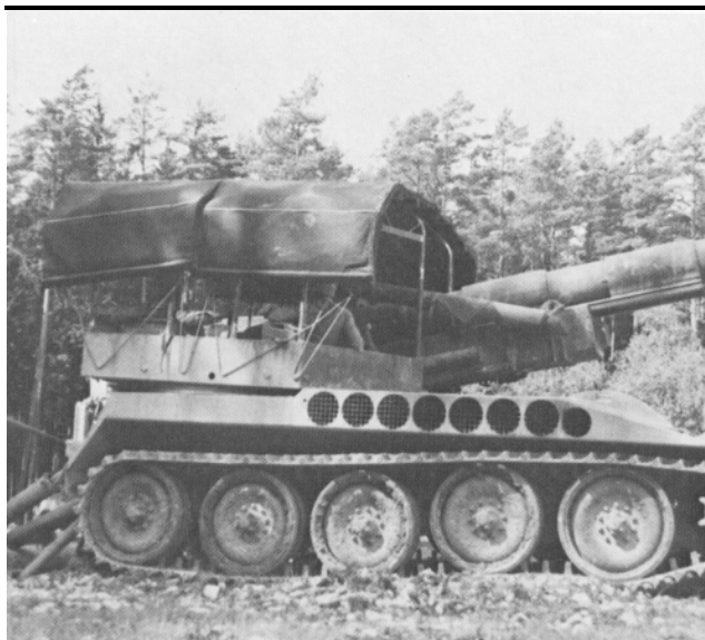
A new canopy being tested by the 41st Field Artillery Group will protect crewmen from the shrapnel of incoming rounds landing as close as 50 meters. (Photo by David Beebe)
