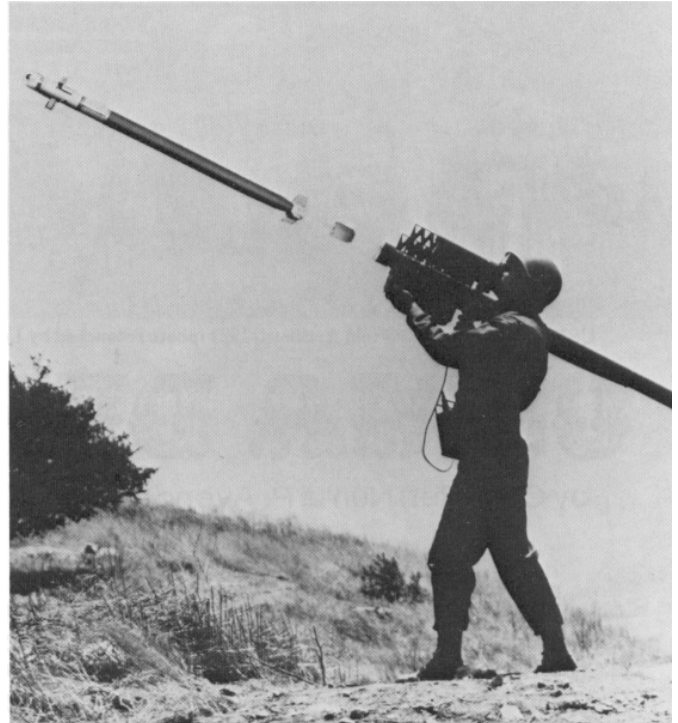
A soldier fires a Stinger missile. Visible between the missile and the launcher is the small ejector motor which propels the missile far enough to prevent blast burns to the gunner when the missile ignites. (Army photo by Frank Ontiveros)
