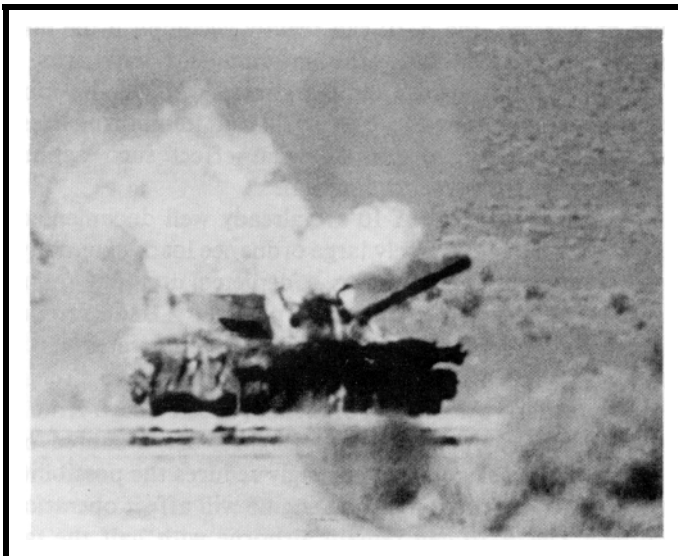
The lethal effects of the A-10's 30-mm GAU-8/A gun system are vividly shown in these two photographs. At left, a Soviet Union T-62 main battle tank bursts into flames after being strafed with a two-second burst of 30-mm ammunition. Numerous secondary explosions were caused by the ignition of the tank's internal ammunition. On the right, the aftermath of the A-10's strike is visible. The tank was assessed as totally destroyed by vulnerability experts from the Office of Secretary of Defense. (USAF photos)
