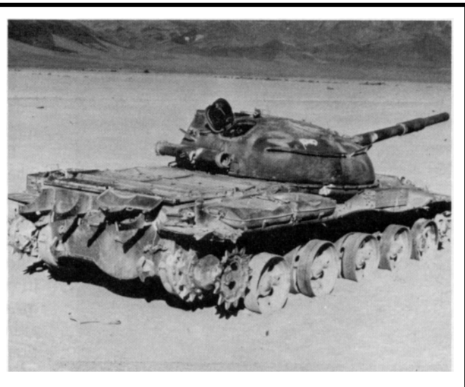
The lethal effects of the A-10's 30-mm GAU-8/A gun system are vividly shown in these two photographs. At left, a Soviet Union T-62 main battle tank bursts into flames after being strafed with a two-second burst of 30-mm ammunition. Numerous secondary explosions were caused by the ignition of the tank's internal ammunition. On the right, the aftermath of the A-10's strike is visible. The tank was assessed as totally destroyed by vulnerability experts from the Office of Secretary of Defense. (USAF photos)
