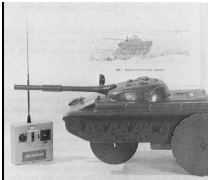
Six miniature moving target (MMT) tanks like the one above are being used for training at Fort Sill's 14.5-mm M31 range. The unit, which resembles a Russian-built T62 tank, was designed by the Army Tank Automotive Research and Development Command. It can travel at speeds up to 1.6 miles per hour in a 600-meter radius from its remote control device shown at left. MMTs have been purchased for use at Fort Sill only, but specifications are available for local Training Aids Service Centers.
