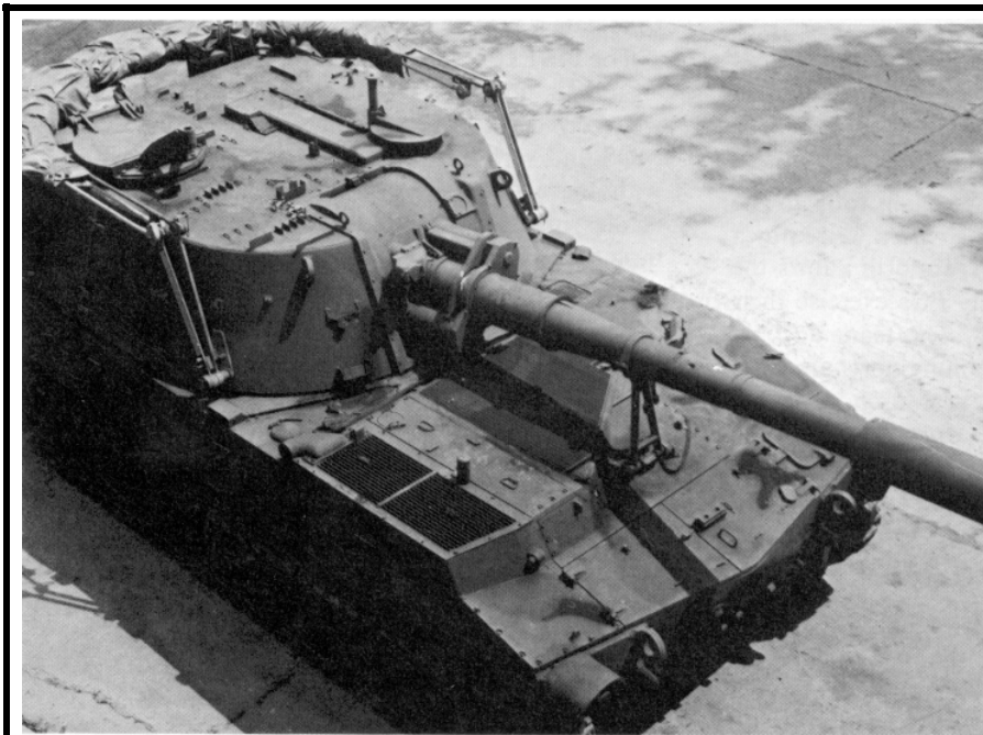
For road march, the canopy is stowed at the rear of the turret. The redesign effort will permit stowage of the barrel disrupter and front and side support structures in this same area.
