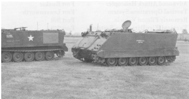
M113A1 normal version, left and stretched version, right.
