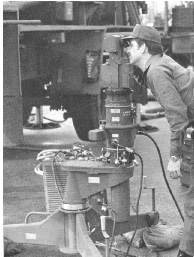
Pershing crew member checks azimuth reference unit of new ARS/SLA ground support equipment. Reference unit uses a laser beam in an automatic optical link to align missile gyro with true north, thus eliminating the requirement for launch from pre-selected and surveyed points.
