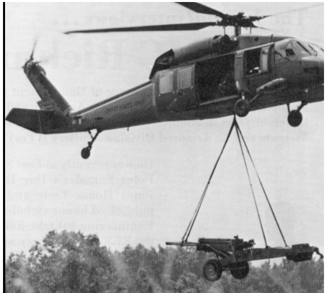
The UTTAS, shown here lifting a 105-mm howitzer, can lift an external load of 8,000 pounds at lower altitudes.
