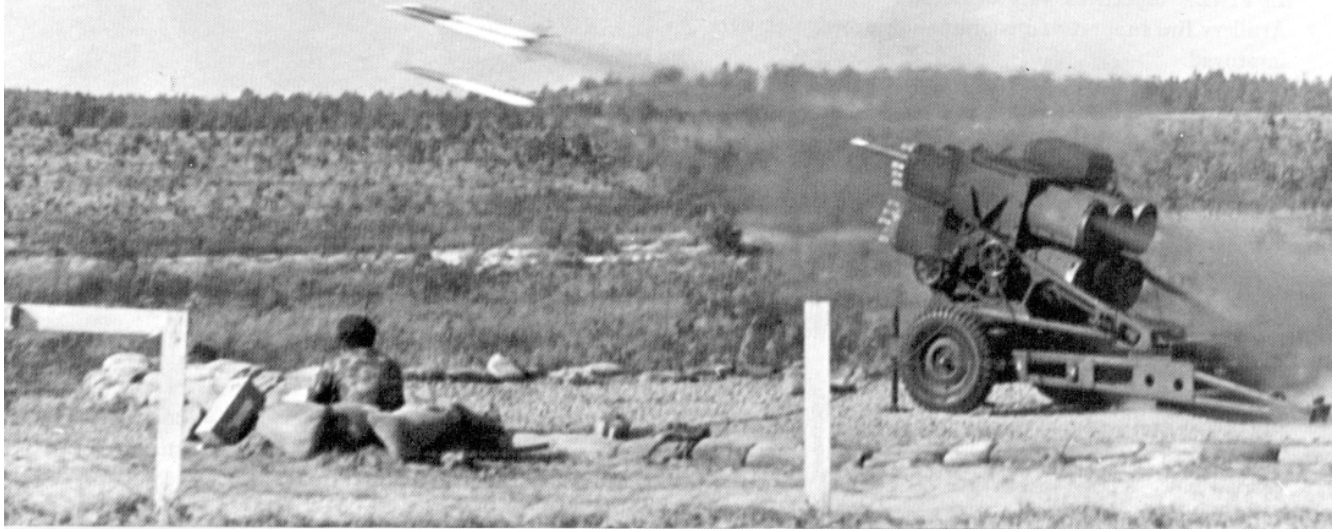
Adjusting rounds being fired from SLAMMER. Rockets can be fired singularly or in groups.
